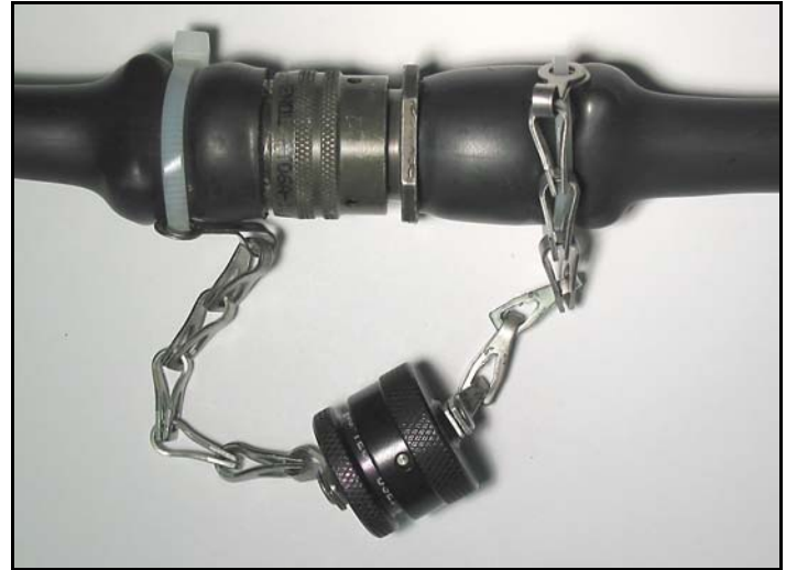
Fig. 2-3: Cables joined with military-grade cylindrical connectors and connector caps joined for protection from dirt.
