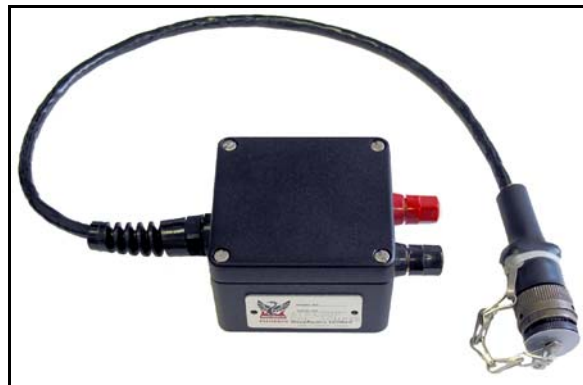
Fig. 2-40: Air-loop CAL Box.
