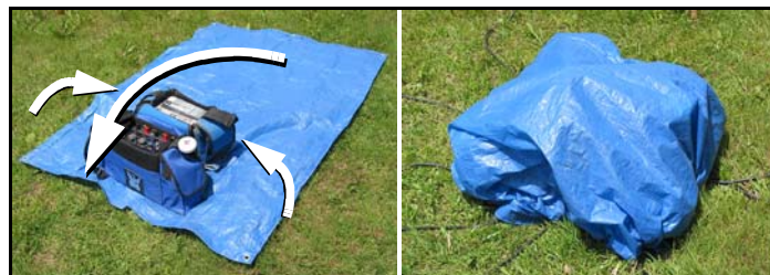
Fig. 2-51: In wet or damp conditions, wrap the tarpaulin tightly.
