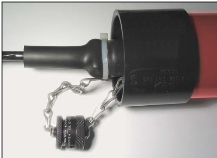
Fig. 2-4: Sensor connector caps joined for protection before burial.
