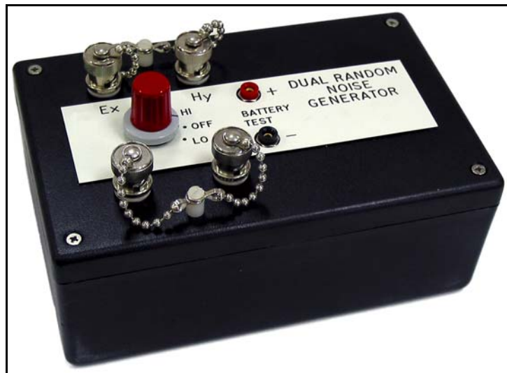
Fig. C-1: WN-2 Dual Random Noise Generator.
