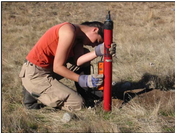
Fig. 2-46: Positioning the coil vertically.
