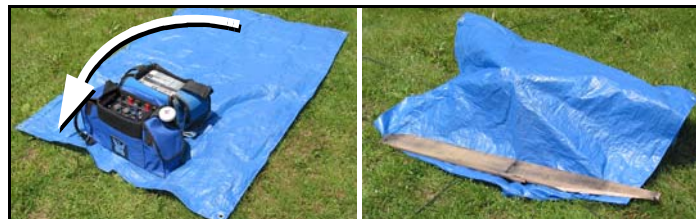
Fig. 2-50: In warm weather, wrap the tarpaulin loosely.
