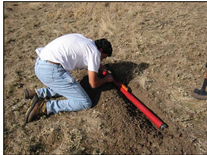
Fig. 2-45: Levelling the sensor.
