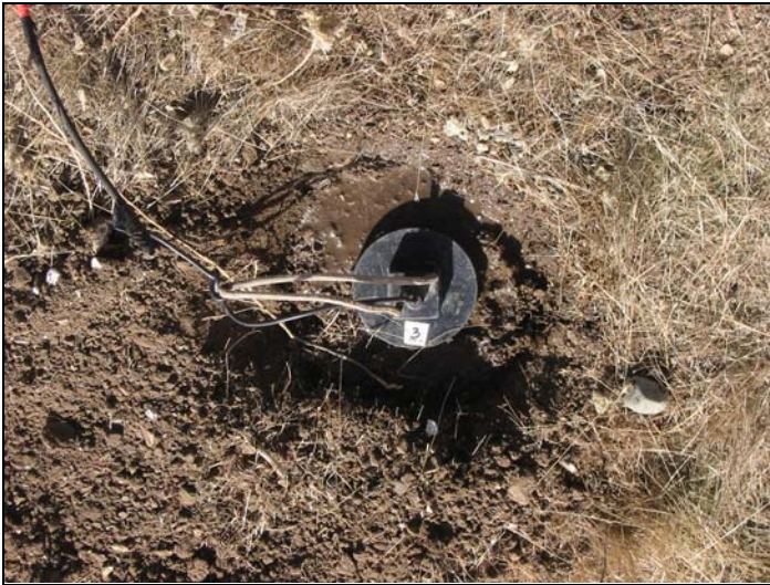
Fig. 2-43: Electrode installed and ready to be covered with dirt.
