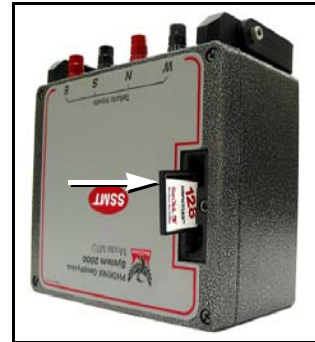
Fig. 2-12: Inserting the CompactFlash card.
