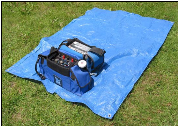
Fig. 2-41: Instrument and battery positioned on tarpaulin.
