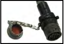
Fig. 2-4: Military-grade cylindrical connector and cap.
