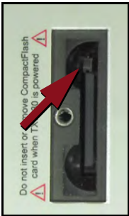
Fig. 2-3: CompactFlash card eject button.
