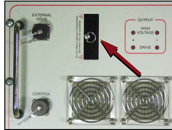
Fig. 2-2: CF card slot on front panel.
