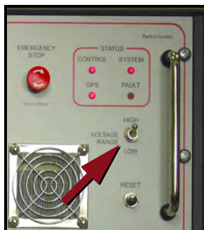
Fig. 4-2: Location of the VOLTAGE RANGE toggle switch.
